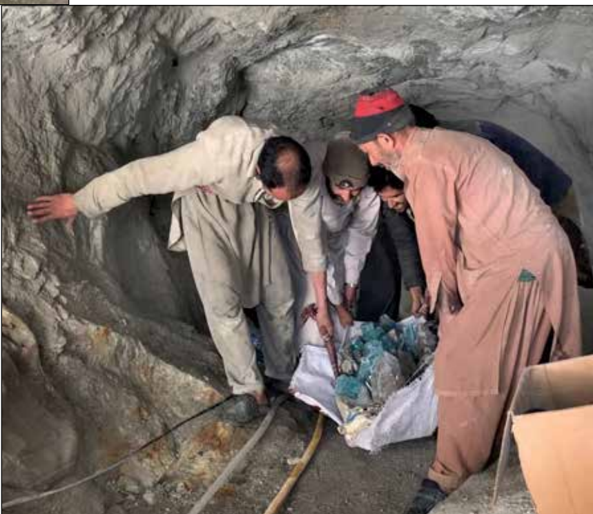
Figure 37. Layers of foam inserted into the pocket for the aquamarine cluster to fall on when it is cut loose from the ceiling. Blue marker shows where the cuts will go. Fine Minerals International photo.
