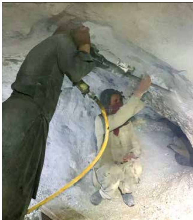
Figure 25. Drilling to cut away the surrounding rock and make a path to the pocket. Feathers and wedges are then hammered into the holes to gently crack the rock. Fine Minerals International photo.
