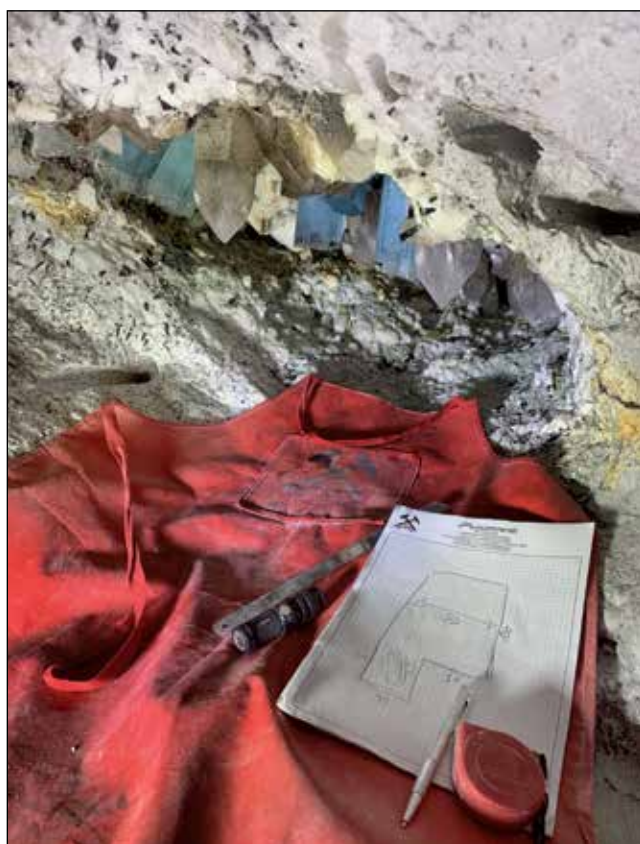
Figure 29. Taking measurements to design an outline for the saw cuts. Fine Minerals International photo.
