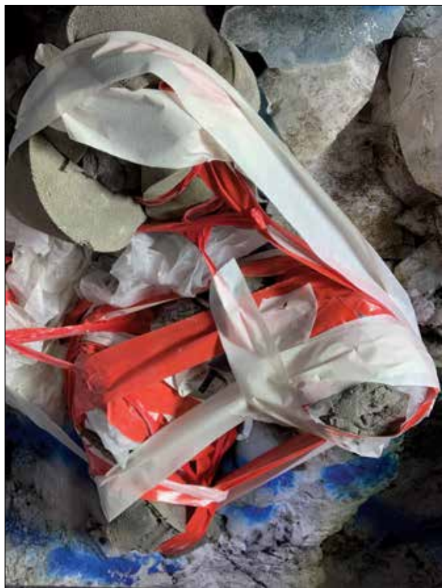
Figure 31. Crystals “bandaged” to protect them during use of the diamond chainsaw. Fine Minerals International photo.
