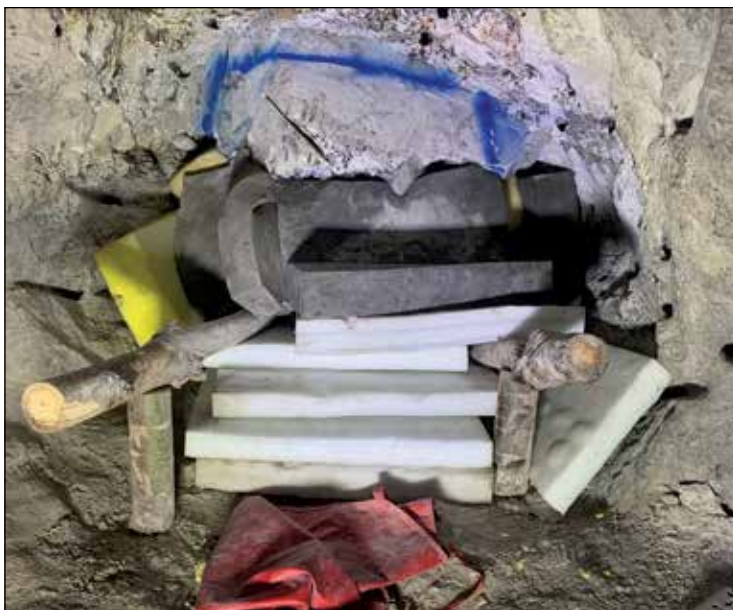
Figure 37. Layers of foam inserted into the pocket for the aquamarine cluster to fall on when it is cut loose from the ceiling. Blue marker shows where the cuts will go. Fine Minerals International photo.
