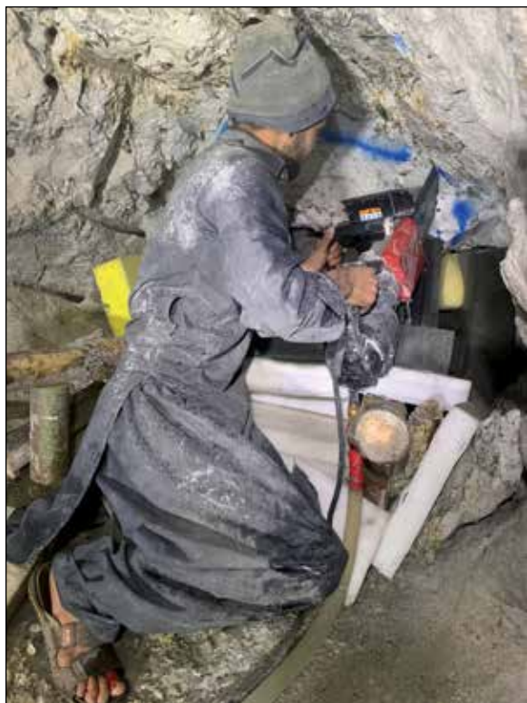
Figure 36. Making one of the final cuts to releasing the King specimen from the pocket ceiling. Fine Minerals International photo.
