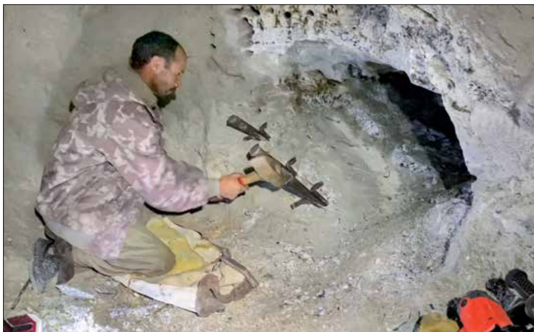
Figure 27. Feathers and wedges being used to break hard rock. Fine Minerals International photo.
